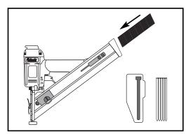
**Figure 1.** Loading the nailer (side view and end view). Match nail heads with head slot for insertion.
